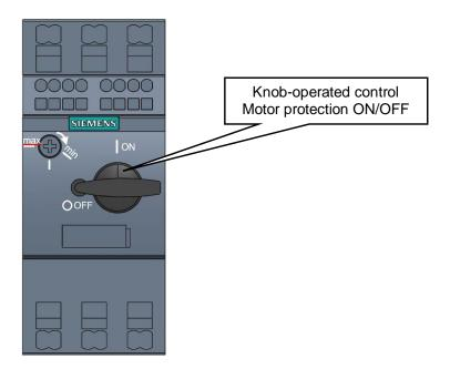
If the consumer is overloaded, the motor protection trips (switch position = 0 Off). This can have various reasons, which should be checked in advance before the motor protection switch is put back into operation via the toggle switch by moving the switch to the I ON position.
