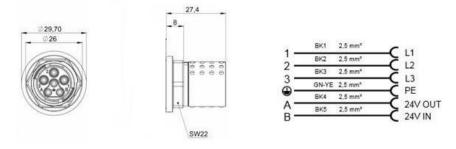
Pin A/B in interface -X20 is used for thermal monitoring of the motor temperature via a bimetal.
