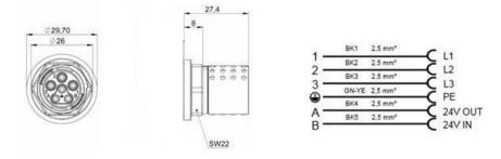
Pin A/B in interface -X20 is used for thermal monitoring of the motor temperature via a bimetal.
